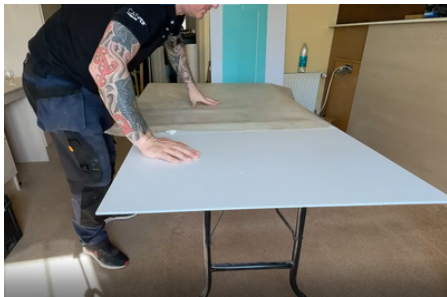
STEP 1 - FIT THE FILM ON FOAMALITE®
